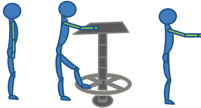
(b) Categorization of hand mode in different standing postures of an agent. Left posture: hand in rest mode , rest mode type: by posture . Middle posture: hand in rest mode , rest mode type: by support , because the hand is lying on a table. The same posture will be categorized as manipulation mode if it would have been without any support as in the right most figure. Right posture: hand in manipulation mode .
