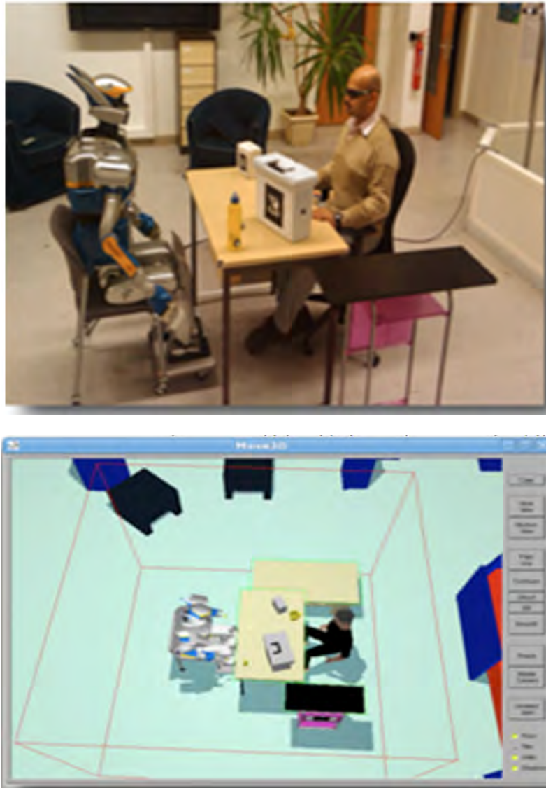
Figure 4.2: Real world and its real time 3D representation in Move3D (see appendix A for detail). The red bounding box shows the current workspace used construct and update the Mightability Maps in real time.
