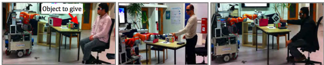
Figure 9.11: (a) Another Scenario for the task of giving an object to the robot. (b) In the absence of any proactive behavior human is standing up and reaching to the robot ( Whole_Body_Effort ) to give the object (c) With proactive reach behavior of robot user is giving the object by only Arm_Effort .
