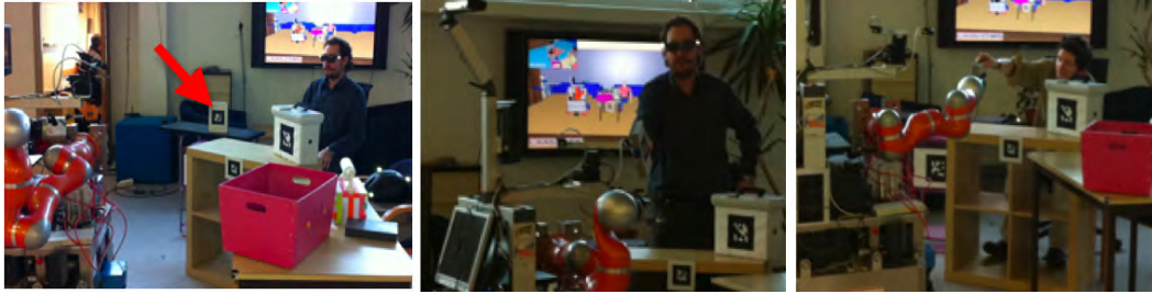
Figure 9.10: (a) Initial scenario for giving the object grey tape marked by red arrow. (b) The human is trying to give by standing up, Whole_Body_Effort , in the absence of proactive reach behavior by the robot. (c) The human is giving just by leaning forward, Arm_Torso_Effort in the case of proactive reach by the robot.
