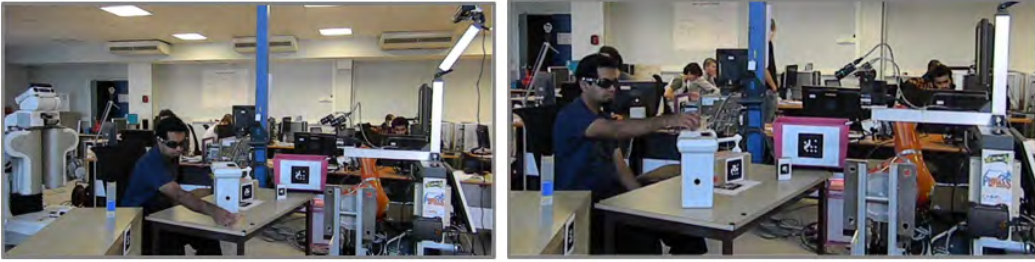
Figure 9.14: The human is making an object accessible to the robot for the initial scenario of figure 9.13. (a) Without proactive suggestion about where to place, the human is putting it close to the robot with Arm_Torso_Effort . (b) With the human adapted proactive suggestion by the robot, the human is now putting it on the white box as suggested by the robot. This has reduced the human's effort to Arm_Effort .
