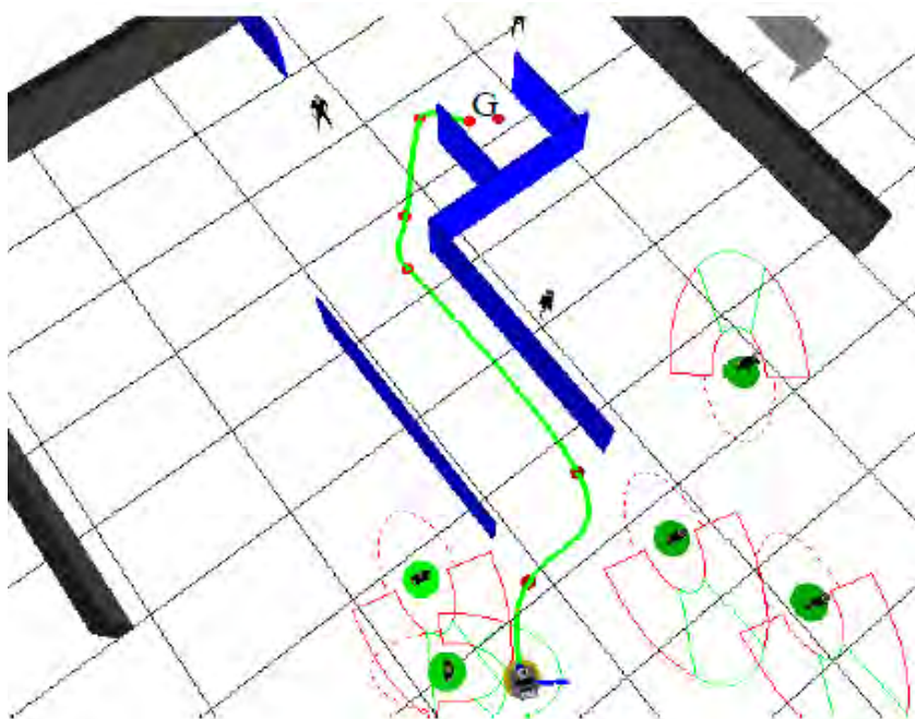
Figure 6.13: Initial socially-aware path generated by the set of social conventions, which are included at time of initial planning. Note that the robot maintains itself in the right half portion of the corridor. In addition, the entire path is smooth.
