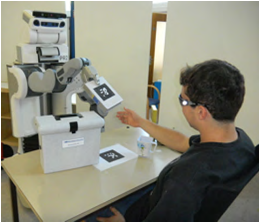
Figure 7.13: Give Task: Maintaining symbolic features , PR2 is giving an object maintaining the object's front towards the human.
