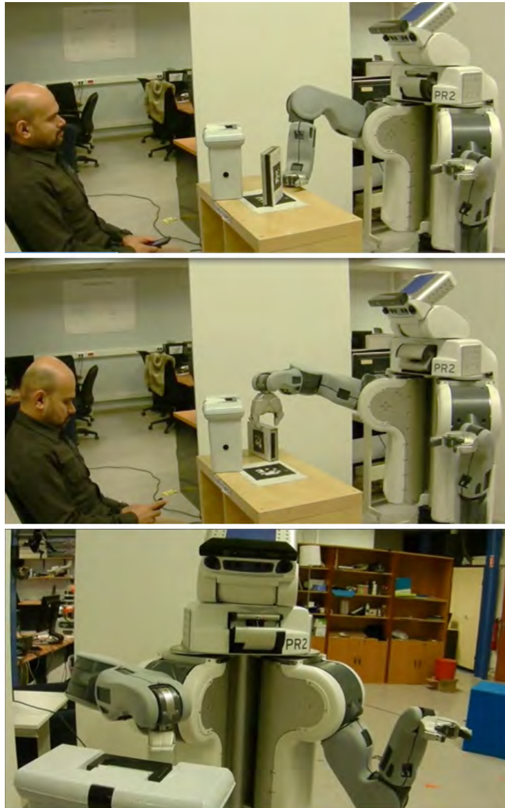
Figure 10.18: Using the effect-to-parameter converter, learnt effects of hide task has been converted into constraints comparable with HRI task planner presented in chapter 7. By using this, the PR2 robot reproduces the task of hiding a target-object (Grey tape) from a target-agent (Human) in a different scenario.
