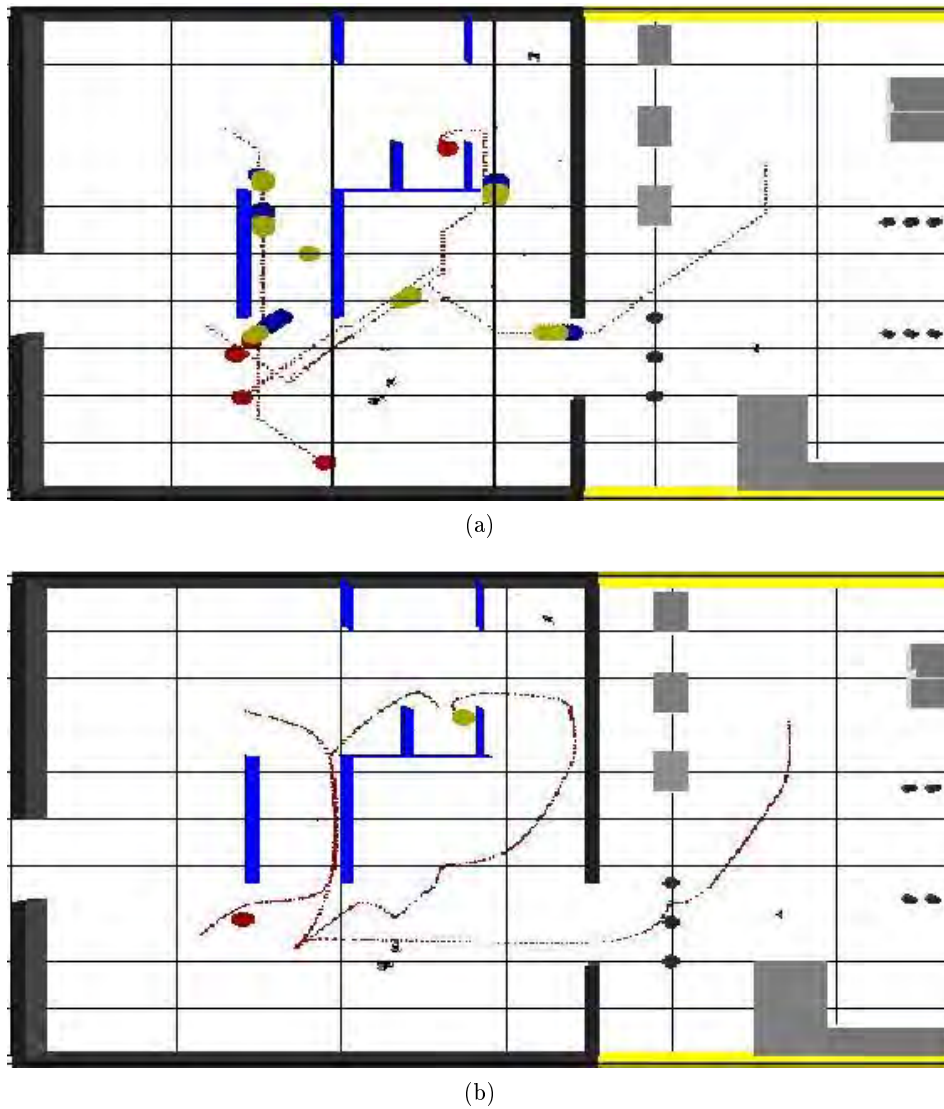
Figure 6.16: Comparing purely reactive behavior based path with socially-aware path: (a) Different clusters of unwanted states (in overlapping blue, red and yellow circular regions along the paths) when navigated by a purely reactive robot (PRR) in the human centered environment. (b) By using our approach of socially-aware robot path (SR), different clusters of the unwanted states has been significantly reduced
