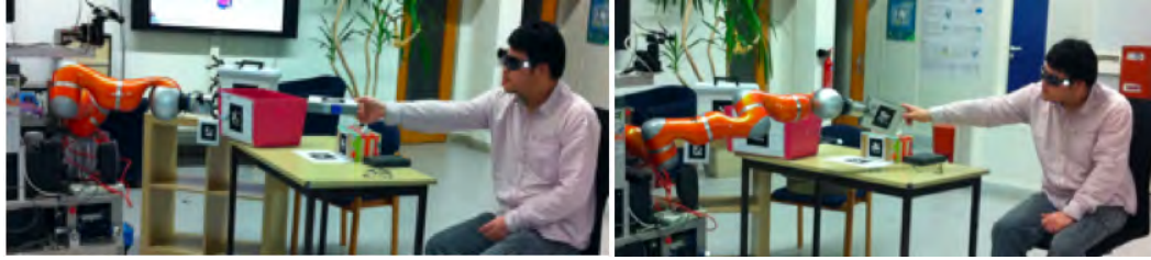
Figure 9.16: Task of giving an object to the robot. (a) In the absence of any proactive behavior the user is holding the object and waiting for the robot to take. (b) With proactive reach behavior from the robot, the user is also putting some effort to give the object to the robot.
