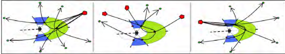
Figure 6.21: Different combination of relative position of the robot (gray circle) and the intermediate goal points (green circles), with respect to the human predicted meeting point, leads to different set of points (red circles) through which the robot should pass during deviation, to show the goal-oriented approaching behavior.
