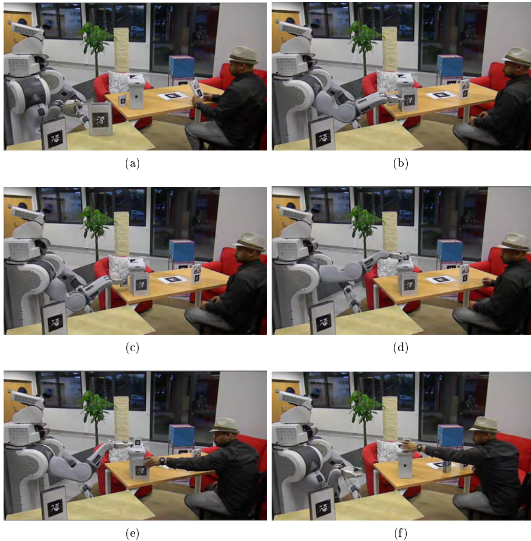
Figure 7.18: Make Accessible Task: Stable placement on the top of other object, ensuring least feasible human effort, (a)-(f): PR2 is sequentially making accessible two different objects to the human, who is sitting in relatively different position than the figure 7.17(a). (a) The first object, which is on the right of the robot is not reachable to the human from his current position and the second object, which is behind the box from the human's perspective is not visible to the human from his current position. (b) The planner autonomously finds a feasible placement for first object. (c)-(d) By taking into account the changes made by its previous action, which leaves no space to place the second object on the table top while ensuring least feasible human effort, the presented framework autonomously finds a stable placement for the second object on the top of the box. (e)-(f) Now the human can easily see both the objects and also take just with Arm_Torso_Effort .
