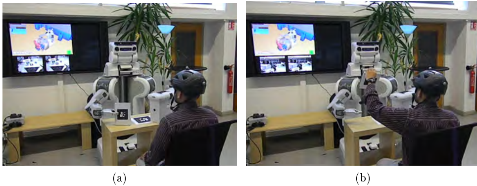
Figure 5.15: Online hand state and mode analyses for another agent’s action. The key facts generated by the system related to the left hand of the agent during the course of action are: (a) Hand in Rest mode , rest mode type: by support , support name: Human , (b) hand in Manipulation mode , hand holding object Grey_Tape .
