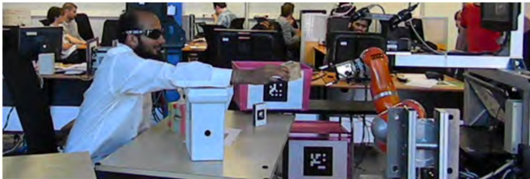
Figure 9.18: Task of making an object accessible to the robot. In the absence of proactive behavior the user is holding the object and waiting for the robot to take.
