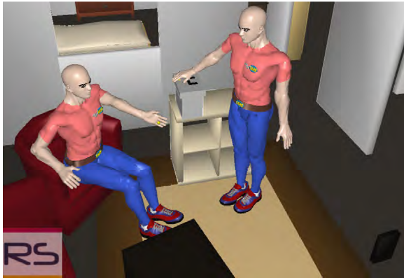
Figure 5.12: Two agents in the environment with different postures and modes of the hands. The system autonomously finds out that the posture of the human on the left is sitting and that of the human on the right is standing . Further, it returns the facts about the agents' hand state: For the left human sitting on the sofa: \langle \text{Righ\_Hand}, \langle \text{Rest\_On\_Support}, \text{Sofa} \rangle \rangle , \langle \text{Left\_Hand}, \text{Manipulation\_Mode} \rangle ; for the right human: \langle \text{Righ\_Hand}, \langle \text{Rest\_On\_Support}, \text{Box} \rangle \rangle , \langle \text{Left\_Hand}, \text{Rest\_by\_Posture} \rangle .
