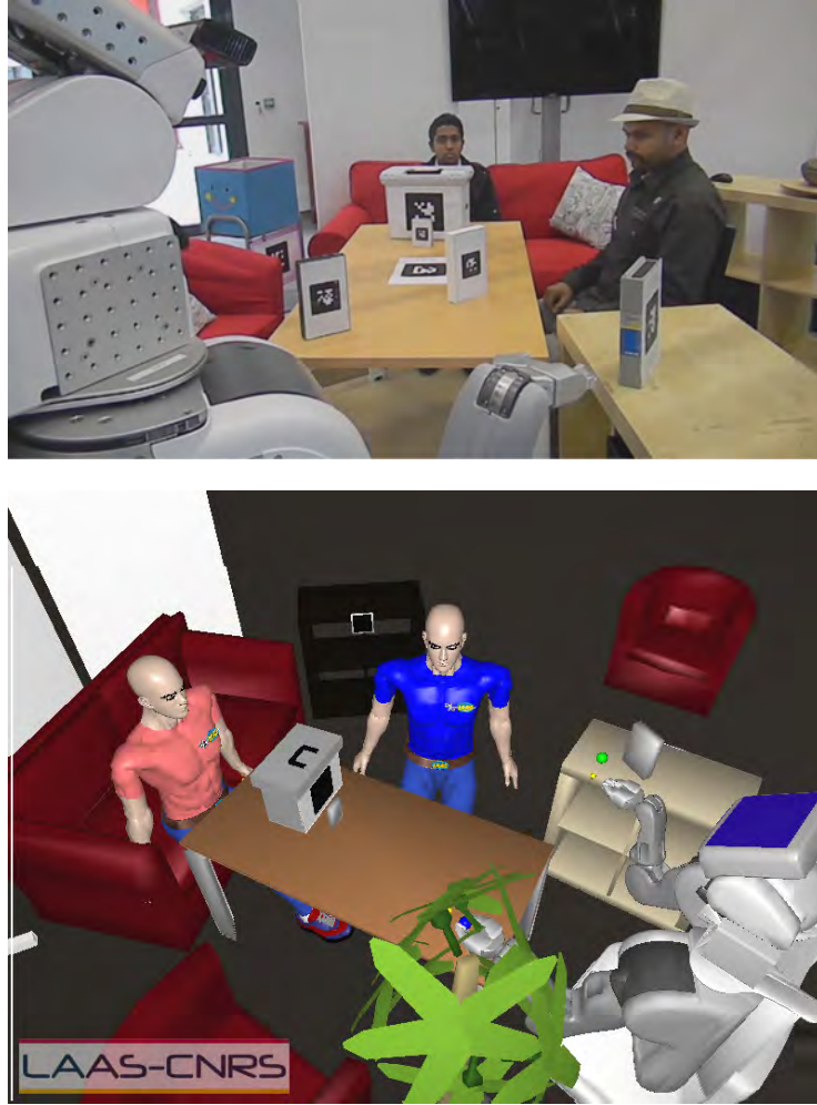
Figure 4.15: Human-Human-Robot interactive scenario (Top). And its 3D model constructed and updated online (Bottom).
