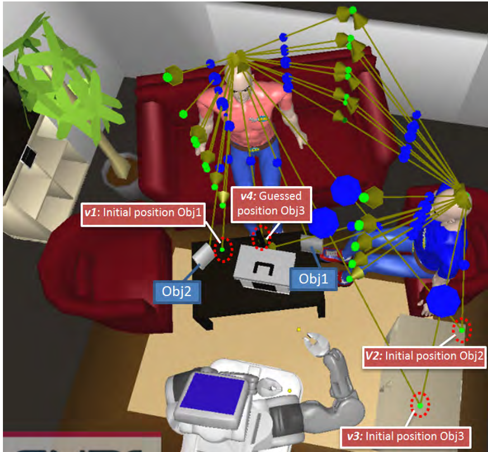
Figure 8.17: Modified affordance graph to ground the changes. Constructed by first introducing virtual object nodes, corresponding to the old positions of the displaced or lost objects in state s_0 in the new state s_1 of the environment and then all the graphs are calculated. For the lost objects, the places where the objects could be hidden are found (by using the agent-agent affordances for hide task) and then one feasible placement orientation of the object is found, which should be making the object invisible to the robot.
