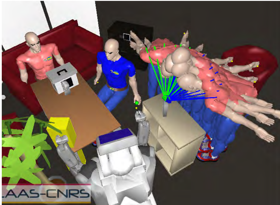
Figure 4.16: Least Effort Analysis for the human currently sitting on the sofa to reach the object on the right of the robot. The robot not only estimates that the human will be required to move but also the possible positions to reach the object; hence, need to put Displacement_Effort , followed by leaning forward.
