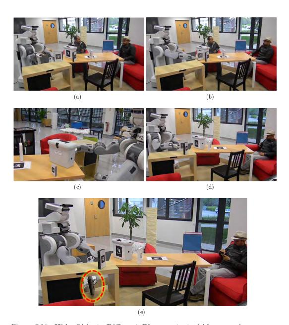
Figure 7.21: **Hide Object**: **Different Placements to hide, ensuring more human effort to see**, (a)-(e) top-down, (a)-(c) PR2 is hiding an object from the human sitting in the middle. Note that as shown in (c) the object is completely hidden from the human's perspective. (d)-(e) Shows the case of hiding the object from the human on the right. The robot has autonomously found a stable placement to hide inside the shelf so that the human will be required to put maximum effort to see it.
