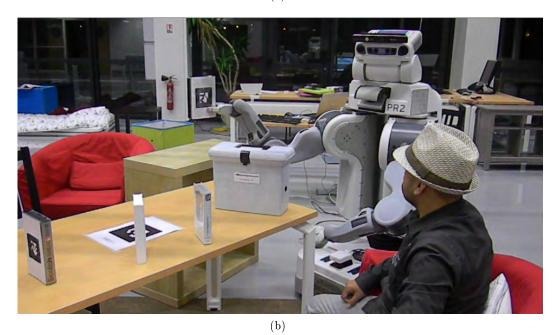
Figure 7.11: Show Object Task: Maximally visible orientation, least human effort, PR2 robot is showing an object, in an orientation to ensure its maximal part is visible and at a place which requires least effort to see the object. Note the difference in final object orientation for different relative human-robot positions.
