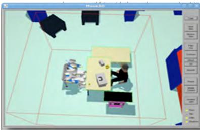
Figure 4.2: Real world and its real time 3D representation in Move3D (see appendix A for detail). The red bounding box shows the current workspace used construct and update the *Mightability Maps* in real time.
