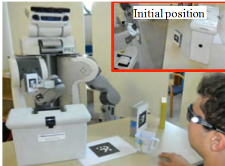
Figure 7.10: Show Object Task: Maximally visible orientation, maintaining object's front and top , PR2 robot is showing an object, in an orientation to ensure its maximal part is visible, while maintaining the front and top of the object from the human's perspective.
