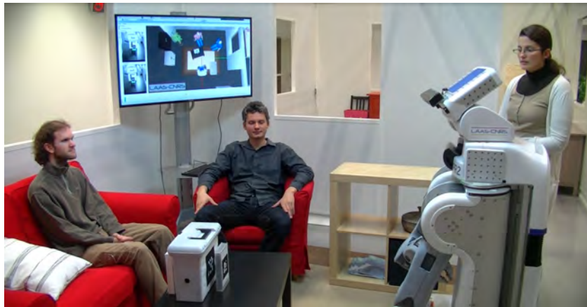
(c) Now the robot is grounding the changes and explaining them. Robot's perception about the current 3D physical state of the environment has been displayed on the TV screen in the figure.
