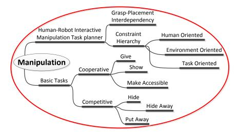
Figure 7.1: Contribution of this chapter: Taking into account *Grasp-Placement Inter-dependency* and introducing *Constraint Hierarchy* based framework for planning basic cooperative and competitive tasks. This chapter identifies and instantiates various key constraints from the perspectives of the *Human*, the *Task*, the *Environment* and the Planning. Another novelty of the framework is to introduce right constraint at right stage of planning to successively reduce the search space.
