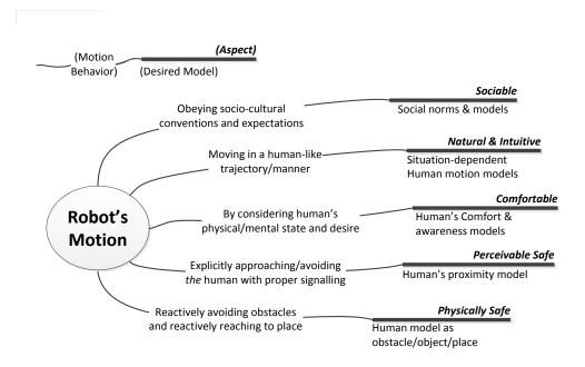
Figure 2.4: We have categorized various factors and qualified the motion aspects, which the robot is expected to take into account while navigating in the human centered environment.
