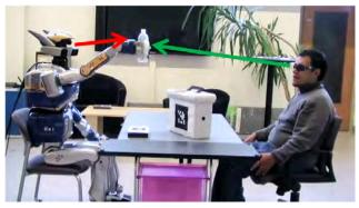
Figure 5.19: The HRP2 robot fetches the human partner's attention in the task of holding and showing an object to the human. (a) While performing the task, the robot first looks at human to *engage* him, then (b) at the object to *draw* his attention.
