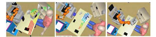
Figure 9.9: Task of making an object accessible by the human to the robot by putting it at appropriate place for the robot to take. (a) Places on the support planes where the human can put the object with least effort. (b) Weighted points where the robot can support the human by taking the object. (c) Robot found the predicted possible placement of the object on the box from where it is feasible for the robot to take.
