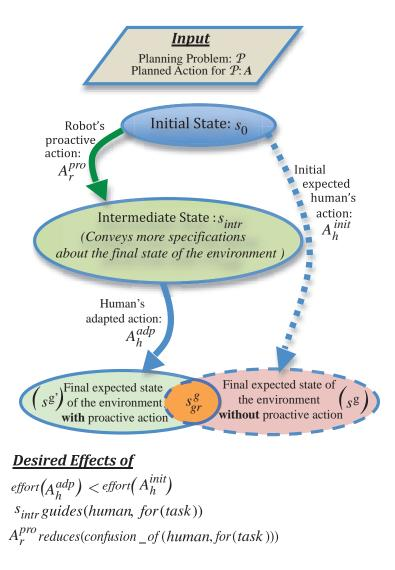
Figure 9.4: A type of proactive behavior, which results into an intermediate physical state of the world and/or changed mental state of the human, mainly to reduce the confusion and effort of the human for smooth execution of the joint task.
