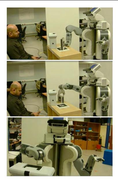
Figure 10.18: Using the effect-to-parameter converter, learnt effects of hide task has been converted into constraints comparable with HRI task planner presented in chapter 7. By using this, the PR2 robot reproduces the task of hiding a *target-object* (Grey tape) from a *target-agent* (Human) in a different scenario.
