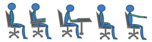
(a) Categorization of hand mode in different sitting postures of an agent. Left posture: hand in rest mode, rest mode type: by posture. Middle three postures: hand in rest mode, rest mode type: by support, because the hand is lying on a support, armrest, table, lap. Right most posture: hand in manipulation mode.
