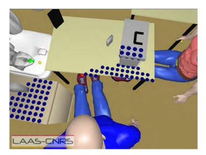
Figure 5.4: Object-Agent Affordance to *Put-onto*: The robot autonomously extracts all the possible supporting objects in the environment. In this scenario, it found that some part of the tabletop as well as top of the box offers the human in the middle to put something *onto* from his current position.
