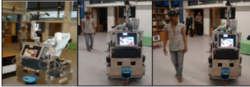
Figure 6.9: The Jido robot avoiding the person by maintaining the social convention of passing by from her left side.
