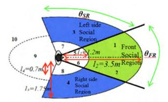
Figure 6.4: Construction of regions around a human, based on proximity and relative position with respect to the human's front.
