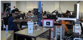
Figure 9.14: The human is making an object accessible to the robot for the initial scenario of figure 9.13. (a) Without proactive suggestion about where to place, the human is putting it close to the robot with  $Arm\_Torso\_Effort$ . (b) With the human adapted proactive suggestion by the robot, the human is now putting it on the white box as suggested by the robot. This has reduced the human's effort to  $Arm\_Effort$ .
