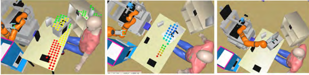
Figure 9.9: : Task of making an object accessible by the human to the robot by putting it at appropriate place for the robot to take. (a) Places on the support planes where the human can put the object with least effort. (b) Weighted points where the robot can support the human by taking the object. (c) Robot found the predicted possible placement of the object on the box from where it is feasible for the robot to take.
