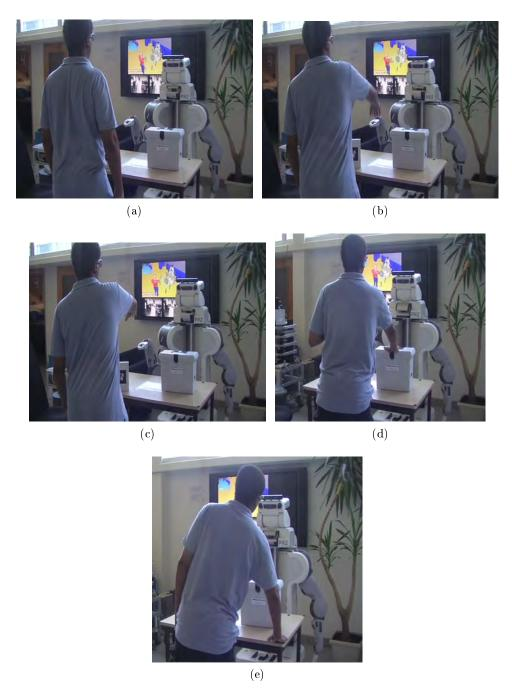
Figure 5.14: Online hand mode analysis for an agent's action. The key facts generated by the system related to the right hand of the agent during the course of action are: (a) Hand in *Rest mode*, rest mode type: by posture, (b) hand Moving, (c) hand in Manipulation mode, hand free of object, (d) hand in Rest mode, rest mode type: by support, support name: Box, (e) hand in Rest mode, rest mode type: by support, support name: Table.
