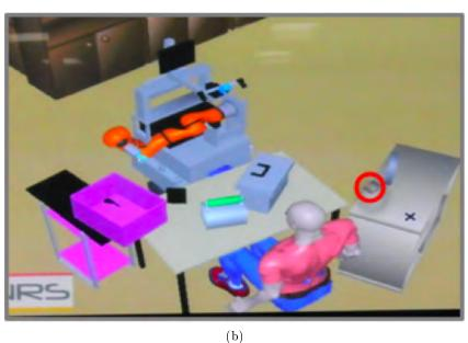
Figure 9.13: Task of making an object accessible by the human to the robot by putting it at appropriate place, so that the robot might be able to see and take it. (a) initial scenario (b) Real time 3D representation of initial scenario, by the robot through various sensors. The object, which the robot will request to make accessible is encircled in red in (a) and (b).
