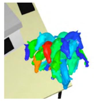
Figure 7.9: Acceptable placement orientations of the toy horse from the human's perspective. Note that in all these orientations, the front is visible and the top is maintained upward from the human's perspective. Blue to Red: Highest to lowest ranking, based on how much part of the horse will be visible.
