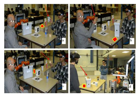
Figure 10.9: Human-Human performing the task to 'show' an object. Initial positions of the *target-object* are shown by red quadrilaterals. (a) Right human is showing the cup by holding it. (b) Left human is showing the wooden cube by holding it. (c) Right human is showing the wooden cube by holding it. (d) Left human is showing the wooden cube by making it visible by putting it on the top of the white box.
