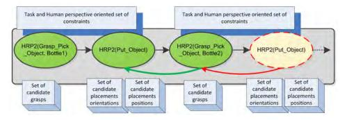
Figure 8.23: Internal representation at geometric level while validating the symbolic plan of figure 8.22. In case of failure to validate 4th node, instead of returning with fail message, the planner backtracks to explore with the alternative to perform the previous actions, so that the current action might become feasible.
