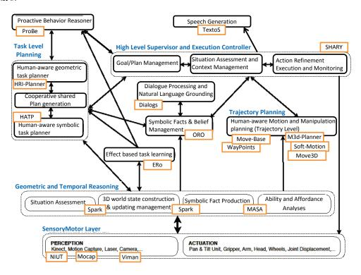
Figure A.1: Main components of the overall HRI system of LAAS and the modules (in orange boxes), which contribute to those components. (Drawing courtesy to Lavindra de Silva, LAAS-CNRS)
