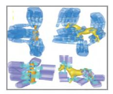
Figure 5.2: Subset of generated grasp set for objects of different shapes, for anthropomorphic hand (top) and for robot's gripper (bottom). (see [Saut 2012])
