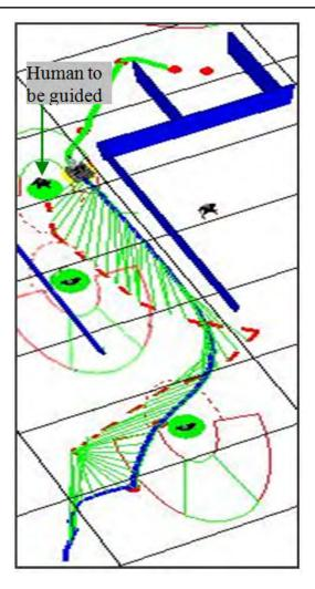
Figure 6.30: Temporal relation between the paths of the human and the guide robot. The robot did not deviate unnecessarily in the case of non-leave taking behavior of the human, hence providing the human with the flexibility to be guided in the way he wants. Note that sometimes the human followed the robot from behind, sometimes he accompanied the robot and sometimes even moved slightly ahead of the robot.
