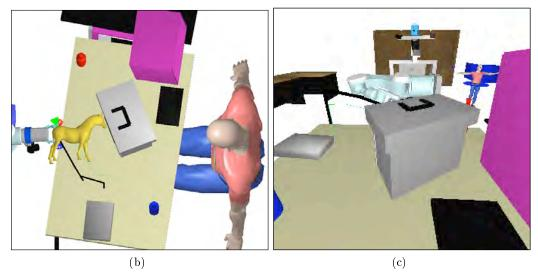
Figure 7.20: **Hide Object Task**: **Grasp-Placement Interdependency**, The planner found feasible object orientation different than its initial one, so that the object will be completely hidden from the human. (a) Initial Scenario, the toy horse is standing upright and visible to the human. (b) The robot puts the toy horse such that it lying by its side. (c) The toy horse is completely hidden from the human's perspective.
