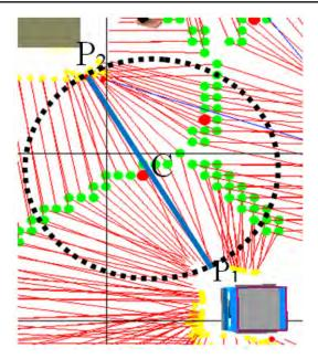
Figure 6.2: Voronoi Diagram based environment clearance analysis. Interesting cell (IC) C and Interesting Boundary Line (IBL)  $P_1P_2$ .
