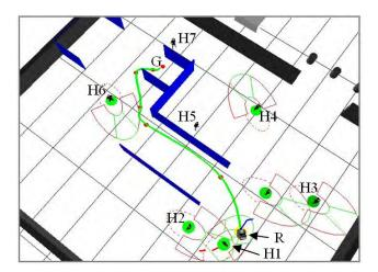
Figure 6.25: The robot JIDO approached the human H1, to start the guiding process. Green path shows the planned path to the goal after the joint commitment of guiding has been established with H1. Note that the initial planned path to guide is also generated using the social planner presented in this chapter, hence, respects the set of social rules.
