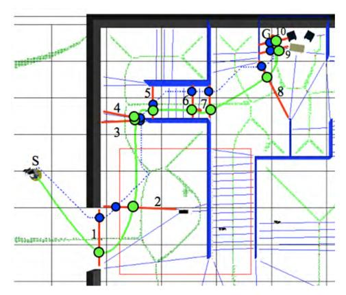
Figure 6.6: Steps of iterative refinements on the path to incorporate social conventions and clearance constraints at planning stage. Blue dotted path from S to G is the initially found  $A^*$  based shortest path. Green path from S to G is the obtained smooth and socially-aware path. Different rules have been incorporated in the different segments of the path by accordingly manipulating the milestones.
