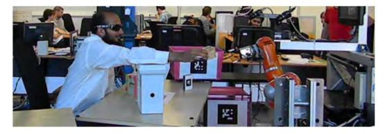
Figure 9.18: Task of making an object accessible to the robot. In the absence of proactive behavior the user is holding the object and waiting for the robot to take.
