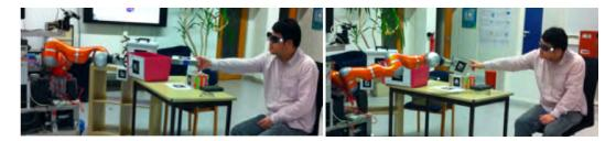
Figure 9.16: Task of giving an object to the robot. (a) In the absence of any proactive behavior the user is holding the object and waiting for the robot to take. (b) With proactive reach behavior from the robot, the user is also putting some effort to give the object to the robot.
