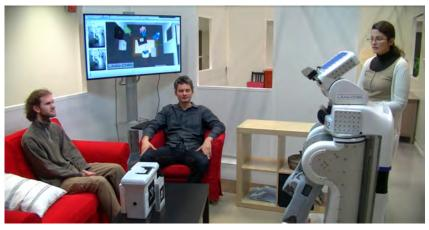
(c) Now the robot is grounding the changes and explaining them. Robot's perception about the current 3D physical state of the environment has been displayed on the TV screen in the figure.
