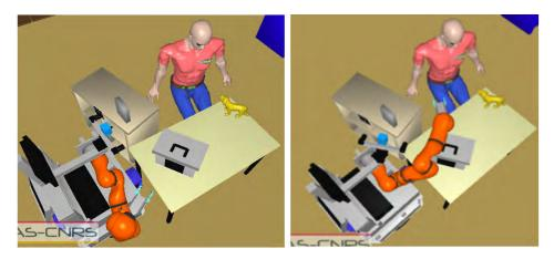
Figure 9.3: Robot asks to the human, "please give me the toy dog." (a) by maintaining its rest position, (b) by proactively moving its hand to appropriate place to guide human's action.
