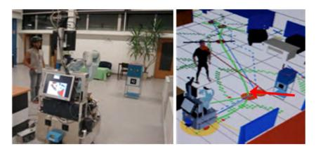
Figure 6.10: The robot crosses a standing person by avoid to enter into her personal space, because no interaction is required. The Red arrow indicates the planned path.
