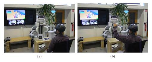
Figure 5.15: Online hand state and mode analyses for another agent's action. The key facts generated by the system related to the left hand of the agent during the course of action are: (a) Hand in *Rest mode*, rest mode type: by support, support name: Human, (b) hand in Manipulation mode, hand holding object Grey\_ Tape.
