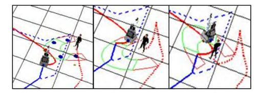
Figure 6.29: The human's re-engagement: The robot predicted that the human wants to join it from its behind so shows no reactive behavior, even if the human is moving in opposite direction of the robot.
