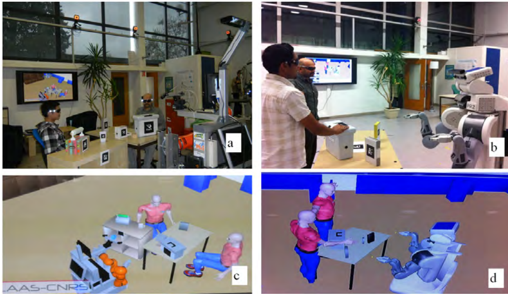
Figure 10.8: Mobile robot JIDO, (a), and PR2, (b), are observing Human-Human interaction scenario. (c) and (d) 3D representation of the world built and updated online by the robots.
