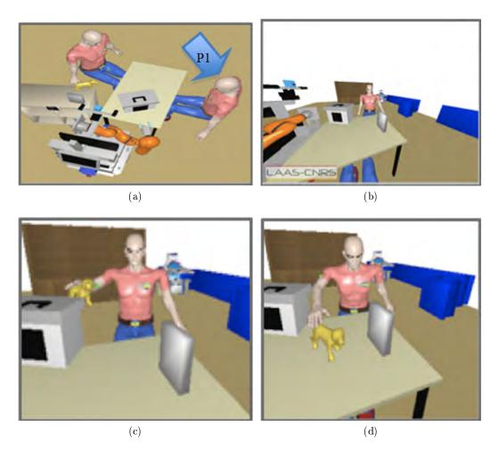
Figure 10.2: (a) The robot is observing a human-human interaction. (b) Person P1's current state visual perspective. Visibility scores of the toy dog for person P1 are 0.0 for the currently hidden toy dog as in (b), 0.001 when the toy dog is partially occluded and relatively far as in (c) and 0.003 when it is non-occluded and relatively closer as in (d).
