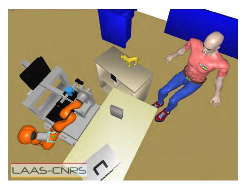
Figure 9.6: Initial scenario in which the human has to give the toy horse to the robot. The robot will plan to proactively reach out to take.
