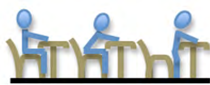
Figure 4.4: Taxonomy of reach actions studied in human movement and behavioral psychology research, [Gardner 2001], [Choi 2004]:(a) arm-shoulder reach, (b) arm-torso reach, (c) standing reach. We have adapted and enriched this taxonomy to develop the human-aware effort analysis table as shown in figure 4.5(a).
