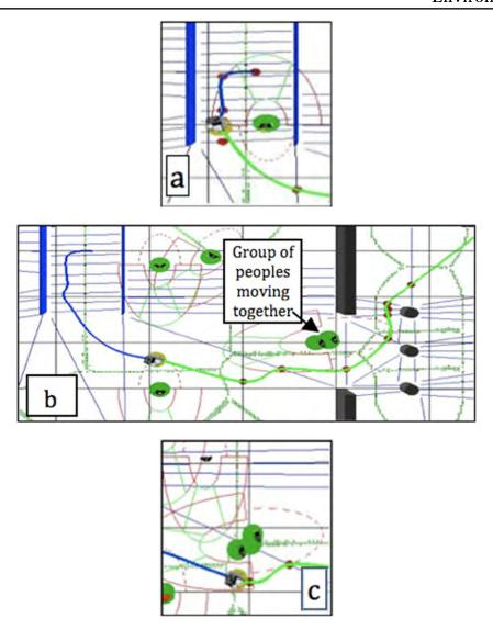
Figure 6.8: (a) The robot is smoothly passing by a person in the corridor, (b) planning a smooth deviation in the path to the avoid group of people with sufficient signaling distance at the expected passing by place (see figure 6.7 for initial path), (c) smoothly and without any conflict, passing by the group from the left.
