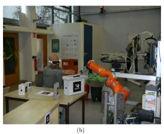
Figure 7.15: Make Accessible Task: Reasoning on the human's effort levels, stable placement on non-table plane, (a) JIDO is picking and (b) making the object accessible by placing it on the white box, so the human can take it with least feasible effort.
