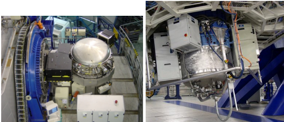
Figure 3.4: Pictures at the left and right panels show the CRIRES and SINFONI instruments mounted at the VLT, respectively.
