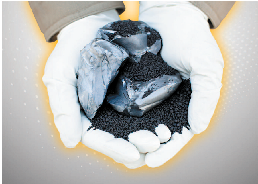
Figure I.2: Photograph of silicon granules obtained in Fluidized Bed Reactor and silicon chunks obtained from milled silicon rods [REC12].
