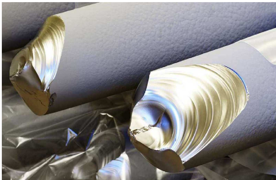
Figure I.1: Photograph of silicon rods obtained through the Siemens process [Pro06].
