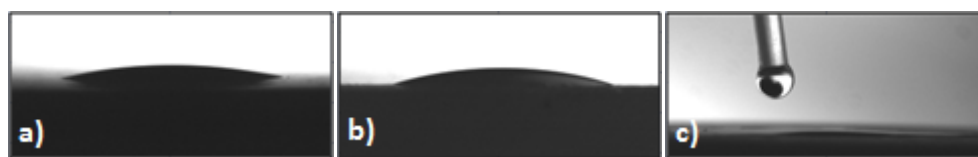
Figure 5. Pictures of acetonitrile droplet deposited on PVDF washed with THF (a); p(VDF-g-PFS) (b), and p(VDF-g-PFS) subsequently modified by MPD (c).
