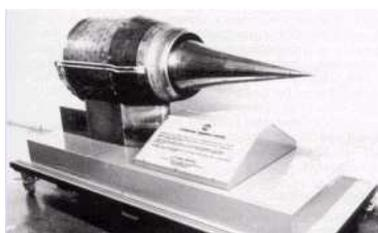
**FIGURE 7.3** – *ESOPE dual-mode scramjet (from [21])*
