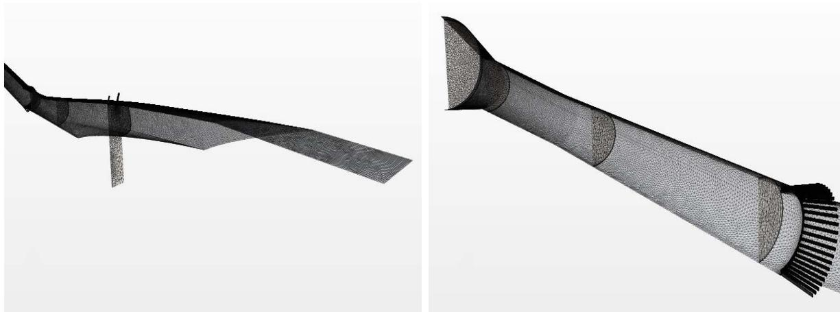
FIGURE 9.1 – Overview of the computational mesh : inlet (left) and combustor (right)
