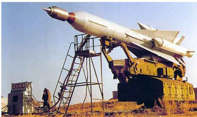
**FIGURE 7.7** – *Kholod mounted on the nose of a modified SA-5*
