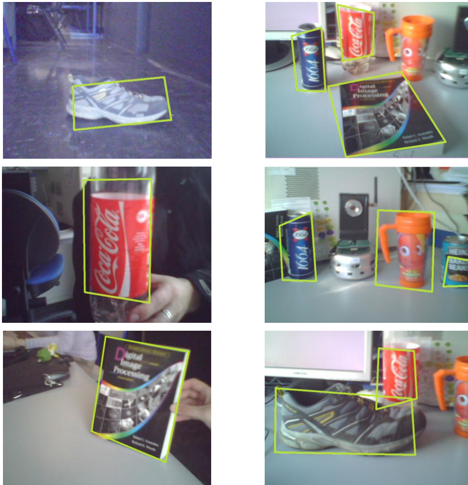
Figure 29: Camera pictures from single (first column) object detection and multiple (second column) previously learned object detection. Successfully detected objects are marked by green lines.
