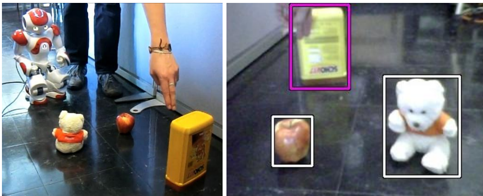
Figure 40: Left: the experimental setup. The tutor is asking the robot to describe the box he is pointing on. Left: the robot's view, with the object in question detected. The robots response was “It is yellow”.
