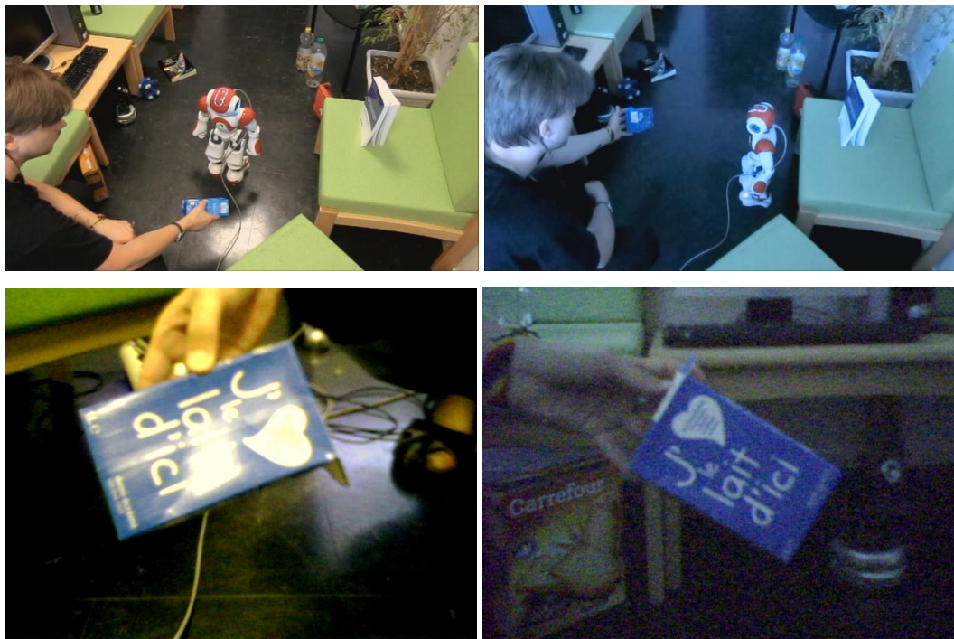
Figure 55: Two different illumination conditions applied while the robot was searching for the same object. Top: external view on the environment. Bottom: robot's proper view through the camera. Left: direct artificial illumination (causing reflections). Right: Natural ambient light illuminating the room through the window. A cloudy day.
