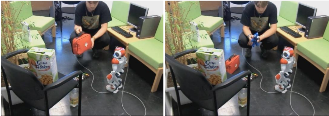
Figure 54: Interaction of the tutor and the robot on subject of things the robot had or had not seen during its exploration. Left: learning the name of a previously seen object (a first-aid-kit). Right: learning the visual appearance and the name of a completely new object (a teddy-bear).
