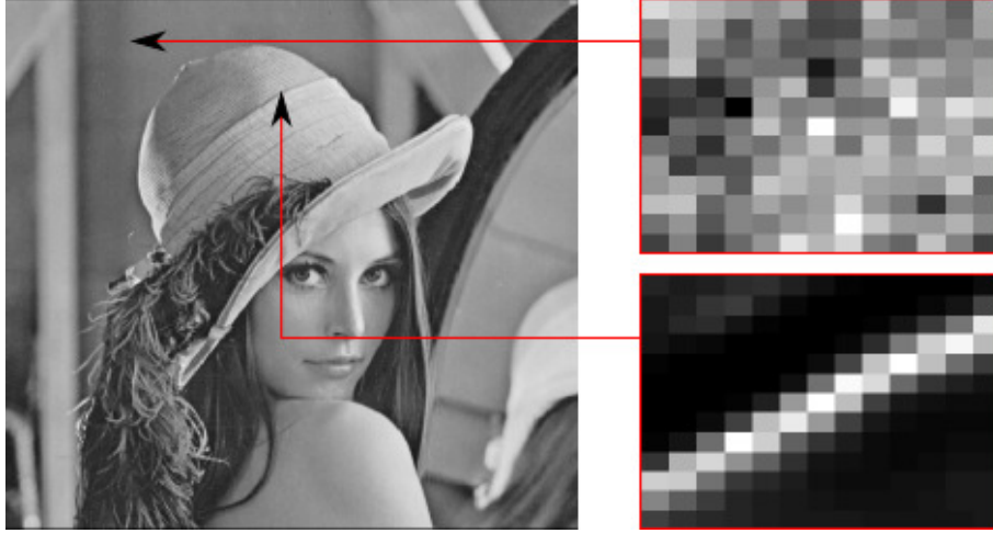
Figure 3.10: Adaptation of the NL-Means kernel to the local structures. The two right images show the kernel weights (\lambda_{i,j,k,l})_{k,l} obtained for a patch in a uniformly regular zone and a patch centered on an edge.
