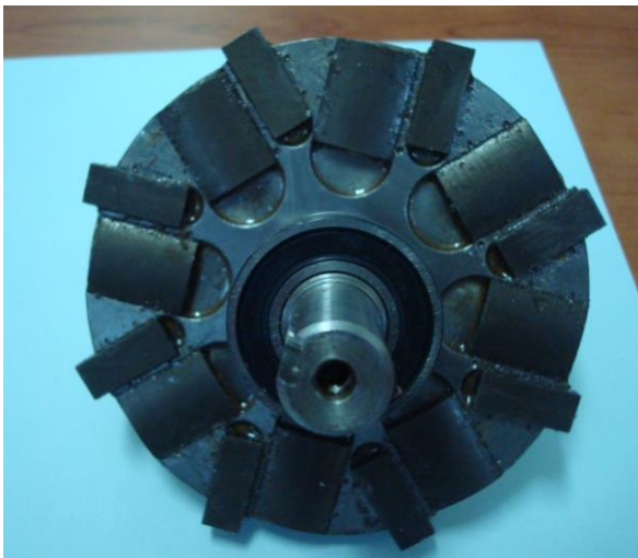
Fig. 1.4. Photograph of the rotor-PM arrangement of the small AFIPM machine built prototype.
