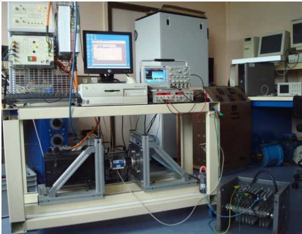
Fig. 4.9. The test bench for the small AFIPM machine in generator mode with resistive load.
