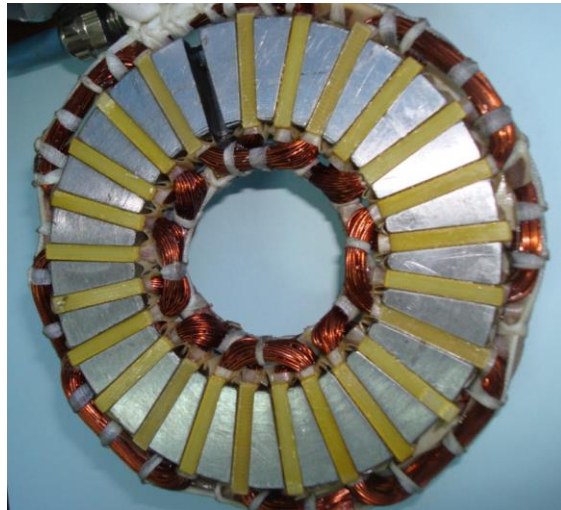
Fig. 1.5. Photograph of one of the two slotted stators with three-phase distributed armature-winding of the small AFIPM machine built prototype.
