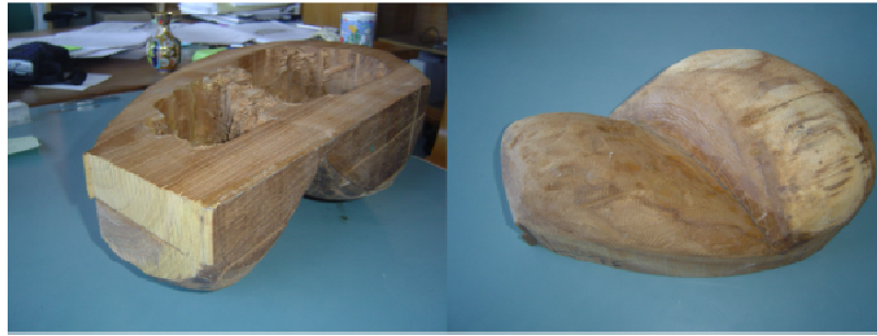
Fig.A.5. Outer and inner parts carved into wood block. Photos from Mr.Zareh's atelier.
