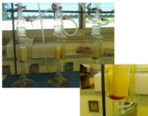
Fig.6.1. Soxhlet system of powder extraction: The color change by methanol can be seen in the picture on the right.
