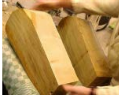
Fig.A.3. Two identical halves of white Mulberry's wood prepared for Târ fabrication (Yousef Pouria's interview. Jadidonline magazine, 16 November 2007).
