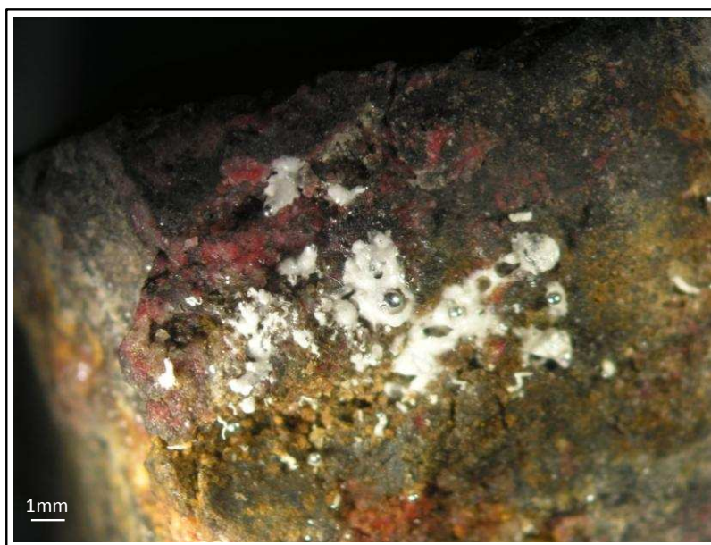
Figure 4.3.: Photograph of a natural ore from Almadén, El Entredicho, showing Hg(0) droplets and the white Hg(NO 3 ) 2 precipitate formed after the application of nitric acid on its surface.
