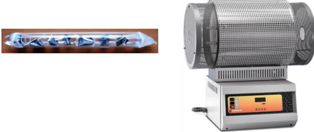
*Figure 2-2: Alloys encapsulated in silica tubes under argon atmosphere (left) and resistance furnace used for annealing (right)*
