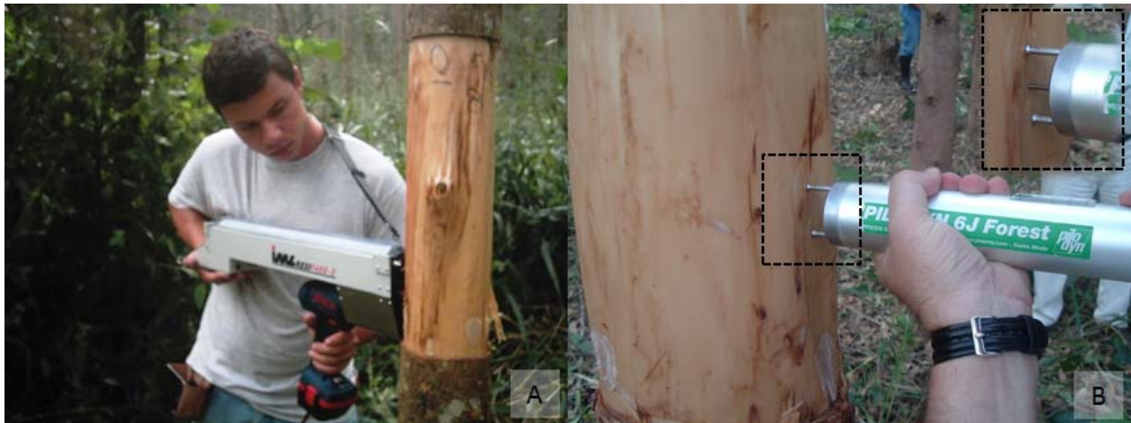
Figure 8 - Evaluating standing trees with Resistograph (A) and Pilodyn (B). Dotted lines shows in detail the pine penetration (source: personal image)
