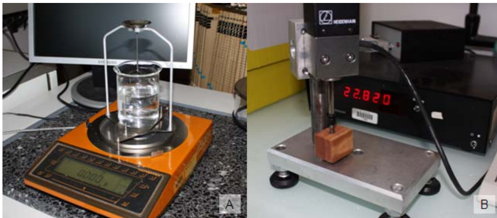
Figure 18 - Experimental dispositive for measuring the green volume of the samples (A) and the sample dimensions (B) (source: personal image)
