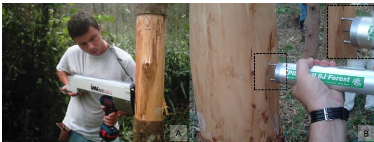
Figure 8 - Evaluating standing trees with Resistograph (A) and Pilodyn (B). Dotted lines shows in detail the pine penetration (source: personal image)
