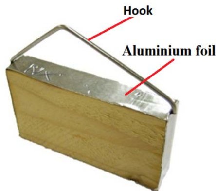
Figure 2.18: Sample used for the measurement of the diffusivity coefficient along one of the principal wood anisotropic direction. The faces perpendicular to the measured direction are sealed with aluminium foil and a hook of iron wire is fixed on the sample.
