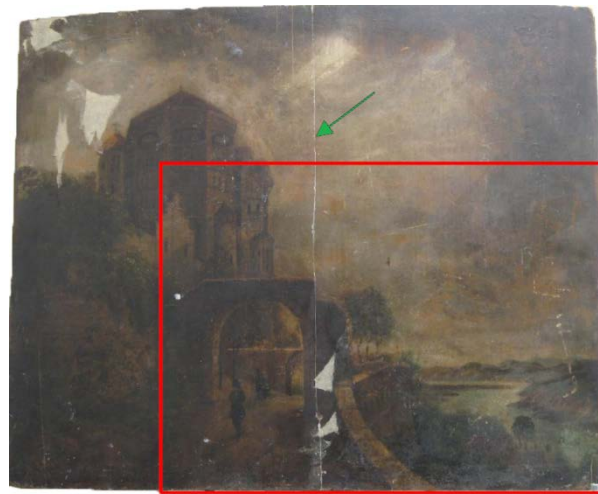
Figure 6.1: The old wooden painting used for cupping measurement. A glue line is clearly visible (green arrow). The red frame indicates the fringe projection measurement area.
