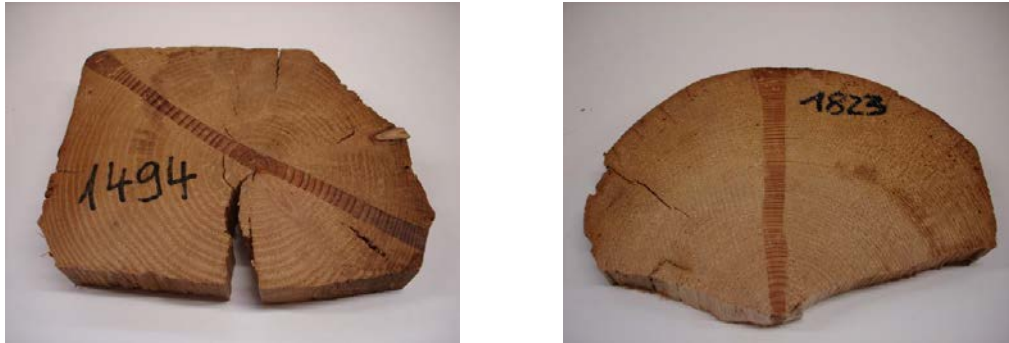
Figure 3.2: Examples of natural aged wood samples dated via dendrochronology.
