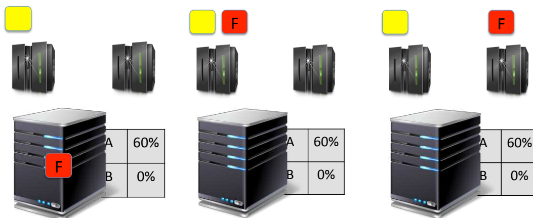
Figure 2.4: Tension between Load Balancing and Deduplication : at the beginning a file wants to be stored, who shares 60% of its content with the chunks stored on node A. If it were to optimize for deduplication, the new file should go on node A, while optimizing for load balancing would imply sending the chunk to node B.
