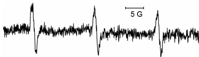
Figure 73: EPR spectrum from spin-trapping experiments with PBN during the reduction of iodo stannatane. Electrolysis at a Pd cathode in \text{CH}_3\text{CN}/0.1 \text{ M TBAPF}_6 , E = -0.7 \text{ V} . T = 293 \text{ K} .
