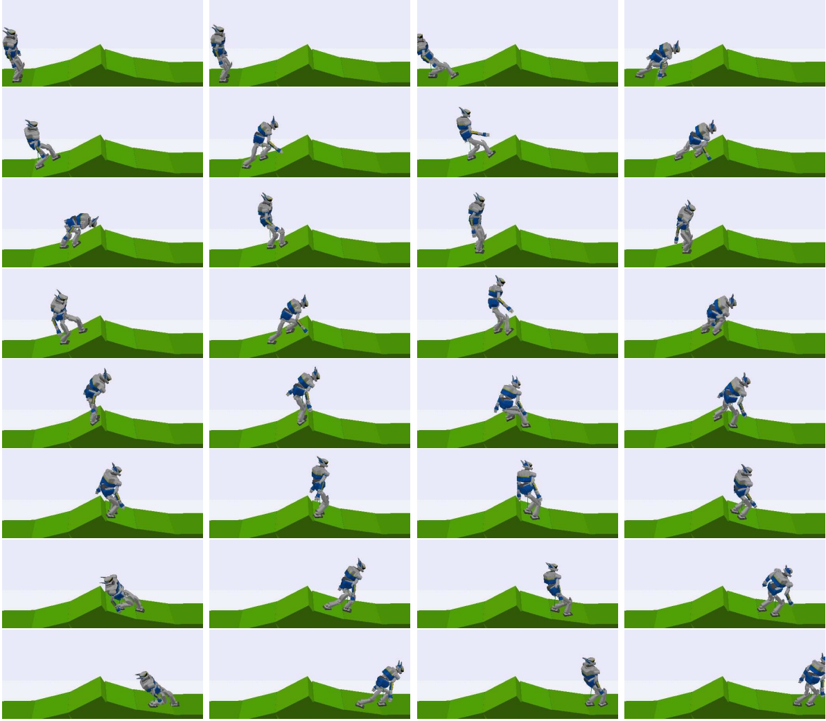
FIGURE 2.5. Biped locomotion over irregular terrain. Coulomb friction allows the robot not to slip. The friction coefficient is set to \mu = 1 .
