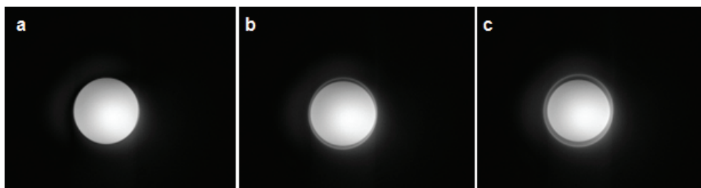
Figure 3.14: Axial images of water-filled syringe acquired in resonance a), and off-resonance conditions corresponding to the frequency shift of fat with respect to water at 3T (440 Hz)(b) and 4.7 T (700 Hz) (c). Acquisition was performed with a bandwidth of 64 kHz
