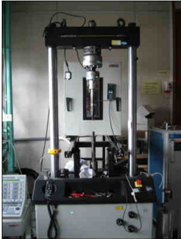
Figure 36 - Machine de traction hydraulique de 10 tonnes.
