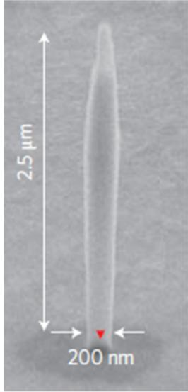
**Figure 2.8: Tapered cylindrical photonic wire** - Scanning electron micrography of a tapered GaAs photonic nanowire containing few InAs QDs. An InAs QD is presented with a red triangle.
