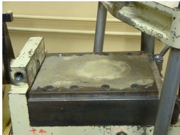
Figure 2.8: Rough surface positioned on direct shear test
