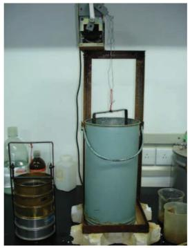
Photo II.1: The Wet-sieving apparatus used in our experiment.
