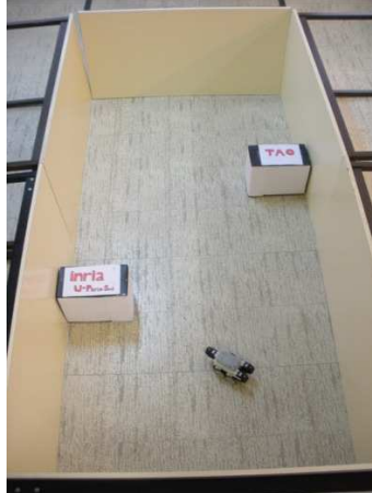
Figure 2.2: The experimental setup used with the real robot.
