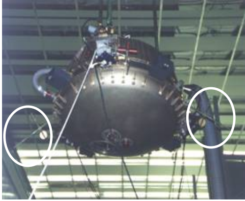
Figure 1 - The Huygens Probe and the two deployable booms (circle marks), where it is possible to observe the set of electrodes.
