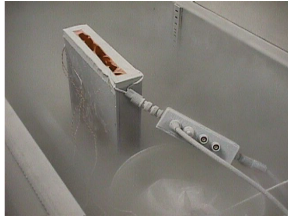
Figure 49: Test equipment for the plate capacitor technique (left) and measurement cell in the thermal chamber (right).
