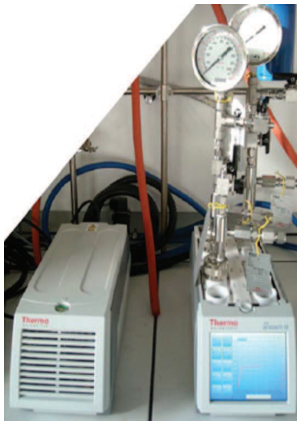
Fig. 1| Picture of autoclave and device use for synthesis of nanoparticles.
