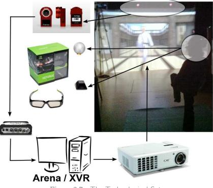
Figure 2.7 - The Technological Setup
