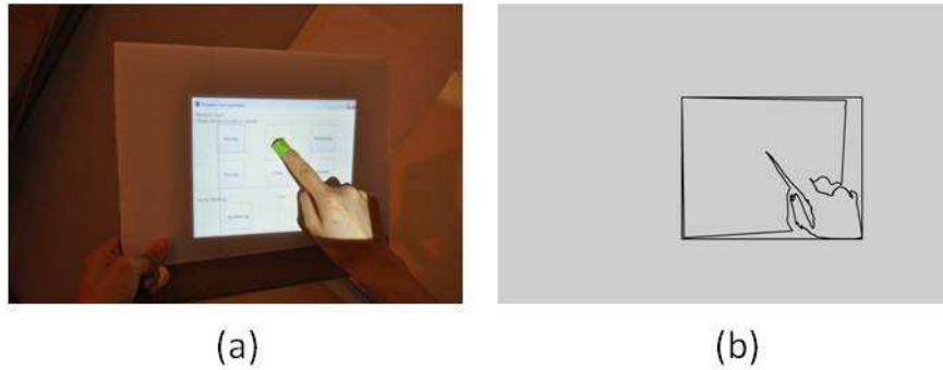
Figure 6.6 The lightest area process. (a). The original projected image. (b). The contour of the lightest area.
