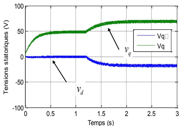
(e) Tension directe et quadrature  $v_{d\_ref}$ ,  $v_{q\_ref}$  (V).
