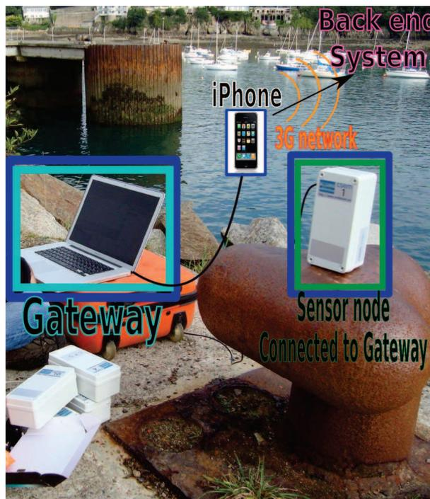
Figure 4.6: An edited picture of the Gateway taken during tests in Brest.
