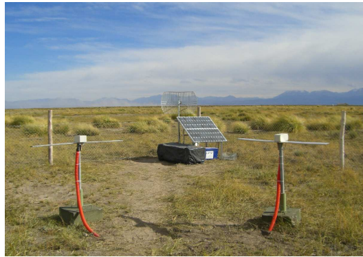
Figure 3. Photo of a radio-detection station with its two dipole antennas and, in the back, the solar panels, the electronics box (covered by a black plastic sheet) and the WiFi antenna pointing toward the CLF.
