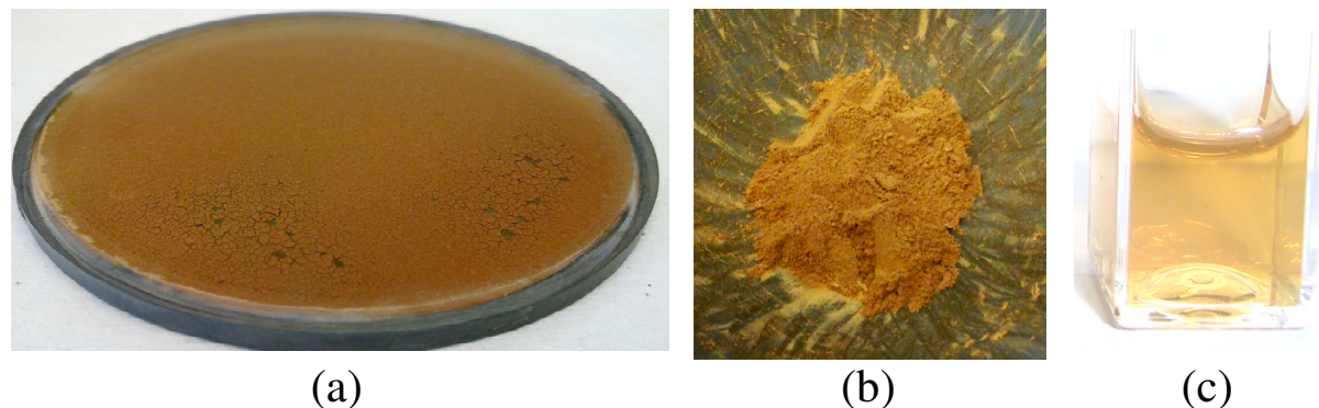
Figure 3.1: Pictures of (a) highly porous 3C-SiC layer, (b) SiC nanopowder, and (c) colloidal suspension with dispersed SiC NPs.
