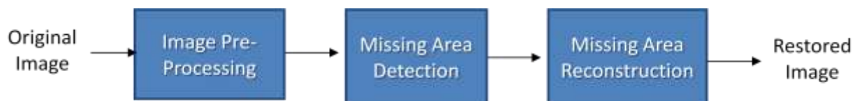
Figure 1.3. General block diagram of an image reconstruction process.
