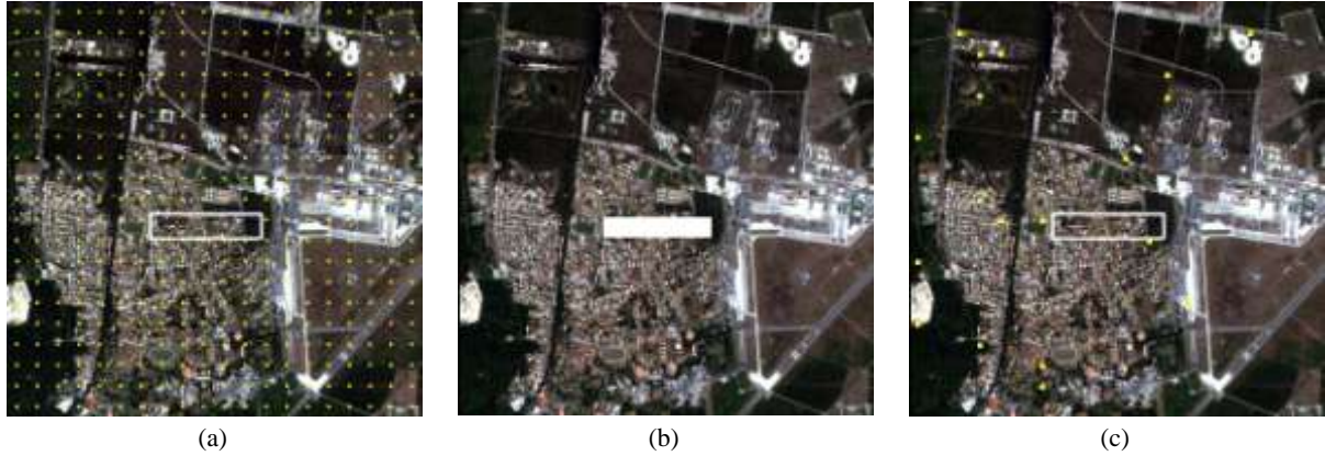
Figure 4.4. ROI A: (a) I^{(1)} image with highlighted TR samples (#TR = 395 samples), (b) I^{(2)} image with the addition of the mask, and (c) reconstructed I^{(2)} image with highlighted SVs.
