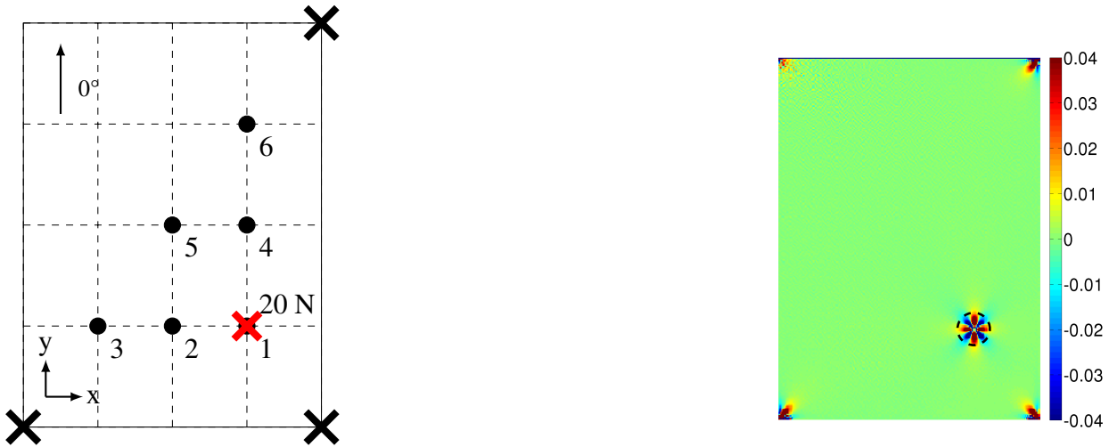
Figure 4.15: EG map for the numerical results from the undamaged sample with 1 pixels sliding pitch and 2 \times 2 pixels 2 sliding window. The dashed circle has a diameter of 5 times the thickness.
