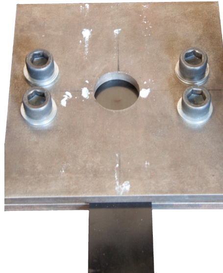
Figure 3.14: View of the top steel plate with the 40 mm diameter cut-out and the sample ready for impact.
