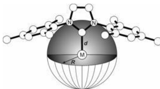
Figure 10. Graphical representation of the sphere used to calculate the % V Bur
