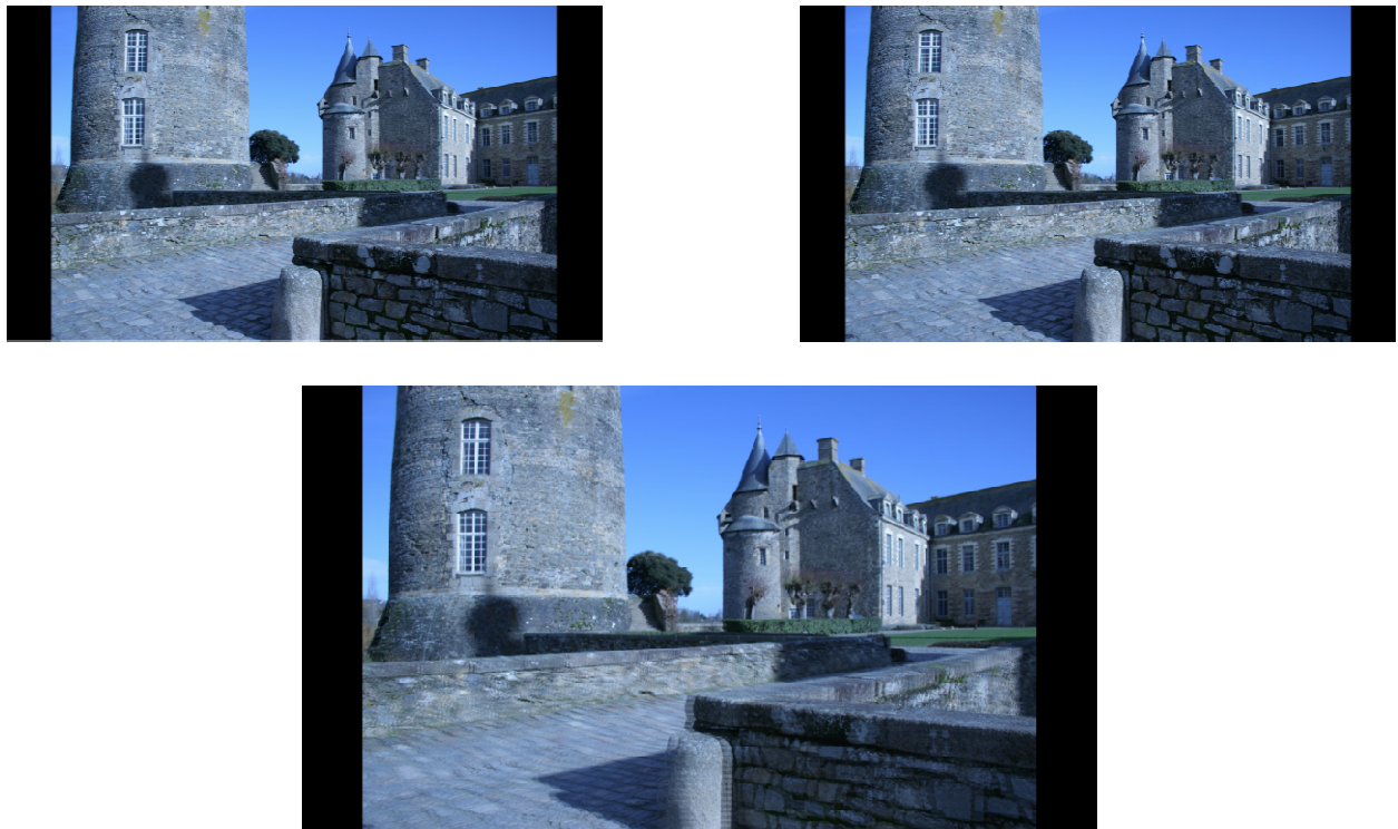
Figure 1.2: How two pictures from slightly different points of view (upper left and right views) give binocular disparity. Upper left and right pictures were taken with a camera baseline of 64 mm, they are here arranged for cross fusion (i.e. left image for right eye and right image for left eye). The lower image is a representation of the two views by interlacing them line-by-line; this method can be used to display 3D content on a polarized display such
