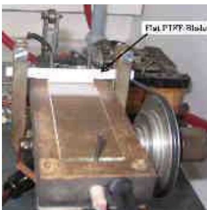
Figure 3-3: Photography of the homemade doctor blade machine. The substrate is placed on the translation bench which can be heated at a desired temperature and moved forwards and backwards.
