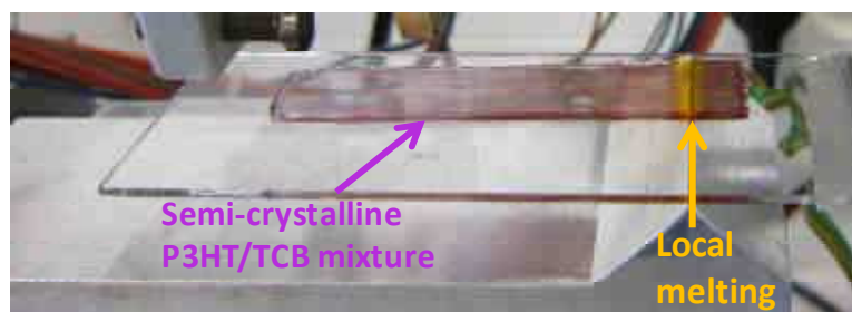
Figure 1-3 : Second crystallization with the local melting apparatus.
