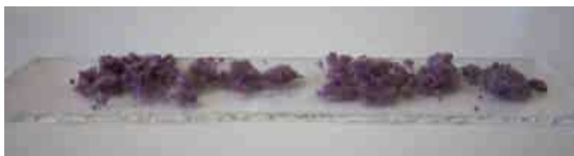
Figure 1-1 : approx. 25mg of the P3HT/TCB powder deposited on a PTFE coated small glass slide
