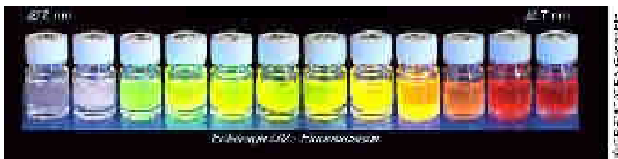
Figure 4-3 : Emission of colloidal dispersions of CdSe spherical nanocrystals with diameters varying between 2 nm (left) to 7 nm (right). Due to the quantum confinement effect, the increase in the size of nanocrystals leads to a red-shift of the photoluminescence from approx. 480 nm to 650 nm.
