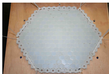
FIGURE 2.24 – Assemblage hexagonal de 217 blocs
