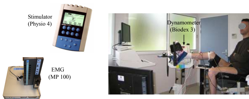
FIGURE 2.4 – Experimental set-up for electrical stimulation and EMG, torque acquisition.
