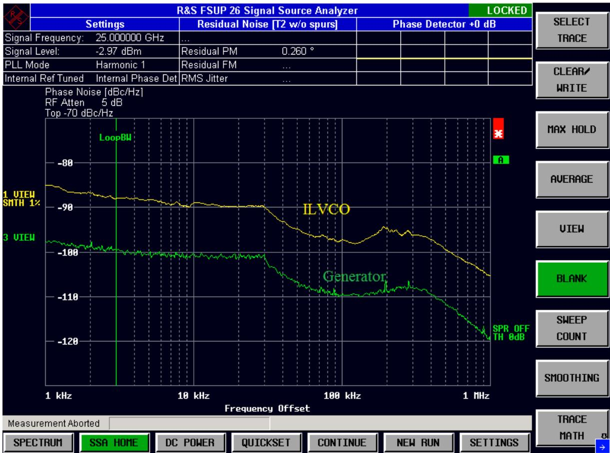
Figure 119: ILVCO phase noise, synchronized on fourth harmonic
