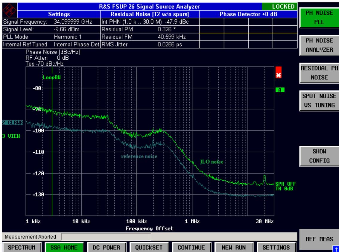
Figure 110: ILO and synchronization signal phase noise (2nd harmonic)
