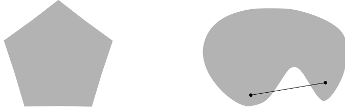
Figure 2.1: Convex set (left) and non-convex set (right).
