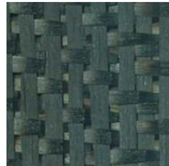
(c) Tissé interlock mince de carbone type 3D (G1151-Hexcel)
