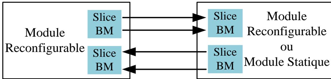
FIGURE 2.6 – Placement d’un Slice bus macro.
